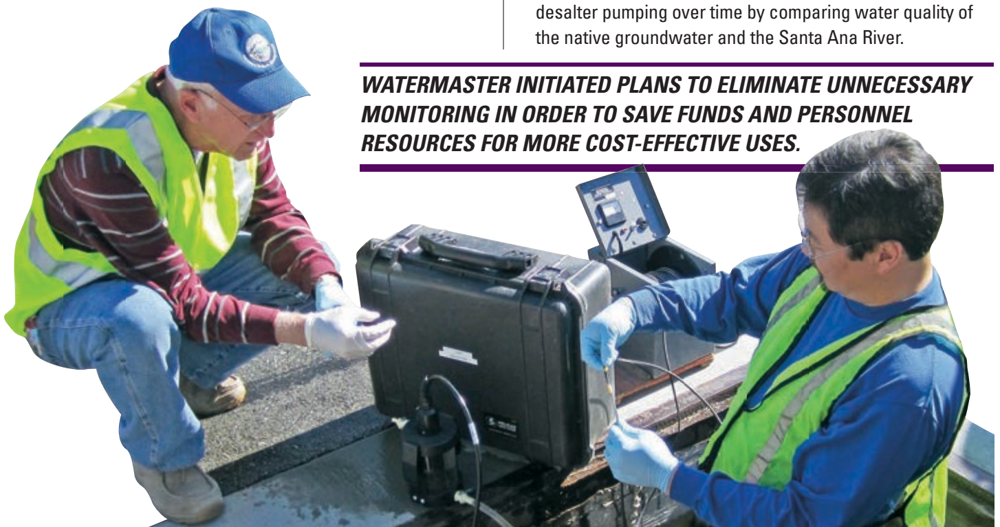
Measuring water quality in a monitoring well located in a street vault in Management Zone 3.
